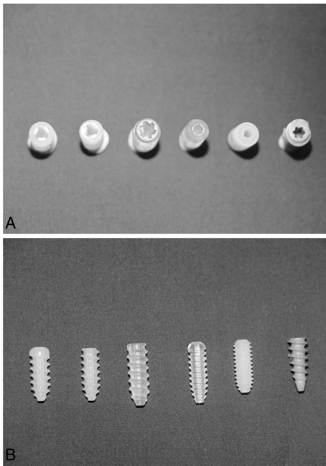
**Figure 1.** Top (A) and side (B) views of the bioabsorbable interference screws tested. From right, Endo-fix, Phantom, Arthrex, Sysorb, BioScrew tibial, and BioScrew femoral screws.
