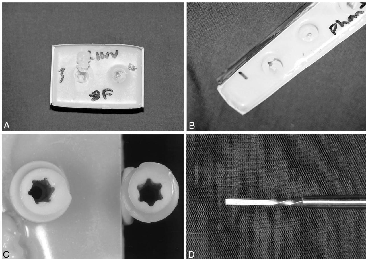
**Figure 2.** Modes of failure. A, mode 1, screw shear at resin-screw interface. B, mode 2, screw failure by splitting radially out from screwdriver hole. C, mode 3, failure of screw-to-screwdriver hole interface. The screw on the left clearly shows the damaged interface compared with the undamaged screw on the right. D, mode 4, failure of screwdriver shaft in torsion.
